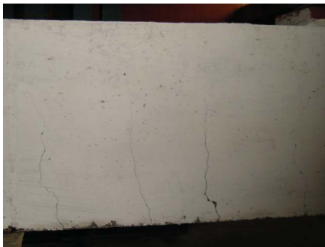
Photo 4 Appearance & Propagation of Crack in the Beam During Fatigue Loading
