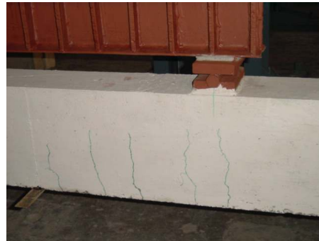
Photo 4 Appearance & Propagation of Crack in the Beam During Fatigue Loading
